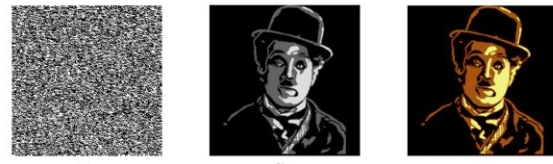
Figure 11. Received GS hologram (a) Demuxed hologram, (b) Reconstructed gray image, (c) Reconstructed color image.
