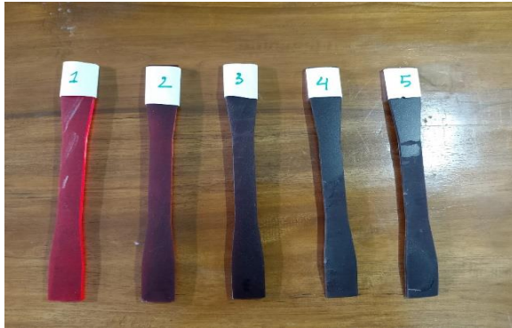
Figure 5. SLA 3D printed specimen prepared with varying compositions of standard resin and CFP (as listed in Table 2).
