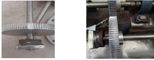
Figure 4. (a) Broken Teeth. (b) Root crack
