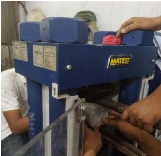
Figure 4. Set up for splitting tensile strength test
