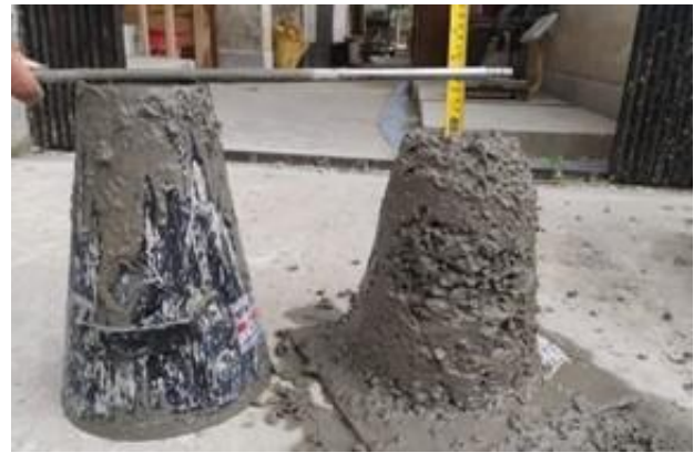
Figure 2. Slump test of concrete.
