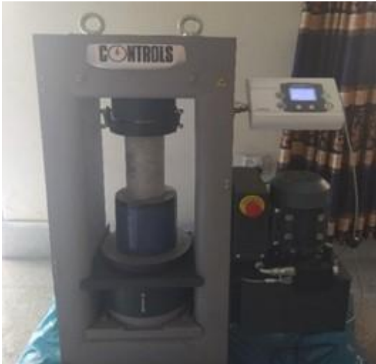
Figure 3. Set up for the compression test of the cylinder.
